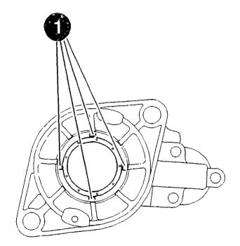
Checking commutator end shield
